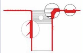
At the mouth of the spigot there are a series of ribs and serrations along the inside, which ensure a leaf guard or gravel-excluder can be fitted into the connector securely.
