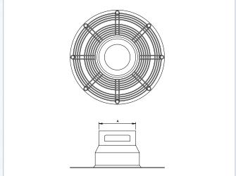
Wallbarn also supplies vents in PVC, for use with compatible synthetic waterproofing membranes. They are designed to aerate the concrete and help the structure to breathe.
