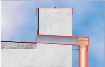
These through-wall units can be fitted to both vertical downpipes at the edge of the retaining wall, or on a horizontal plane through the upstand or wall to connect to the external downpipe.
