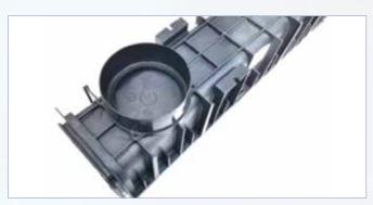
Simply knock the centre out of the moulded connecting bracket on the underside with a hammer and place the connector over the exposed circular hole with the screw holes in the connecting bracket aligned to the holes in the channel.
