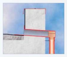
These outlets are available in two versions, with the mouth of the outflow pipe being either 65 x 100mm, or 100 x 100mm for a greater amount of water flow.
