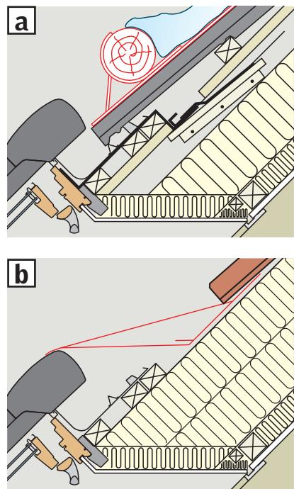
**ENGLISH:** As a precondition to avoiding any damage to the roller shutter in very cold regions and in regions with heavy snowfall, either a snow-wedge or a snow stop must be installed above the roller shutter **a, b**. The roller shutter is protected against overload and will stop automatically if it is blocked.
