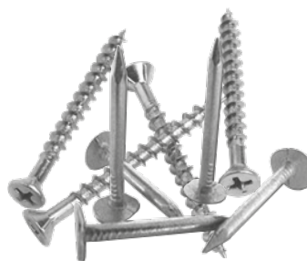
Screws and Nails 30mm screw or nail for tile fitment 50mm screw or nail for ridge/hip cap fitment 75mm to 80mm screw or nail for RidgeMaster/ HipMaster fitment
