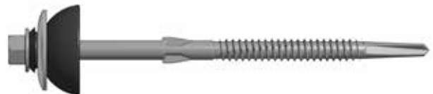
110mm self drilling steel screws for hot rolled steel between 3mm and 6mm - DF12-FCW-5.5 x 60 (80 for vertical).
