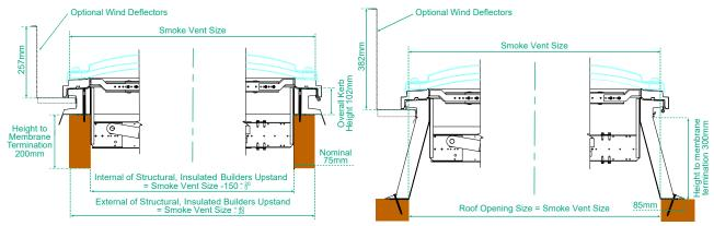
Smoke Vent Fixed to Structural, Insulated Builders Upstand
