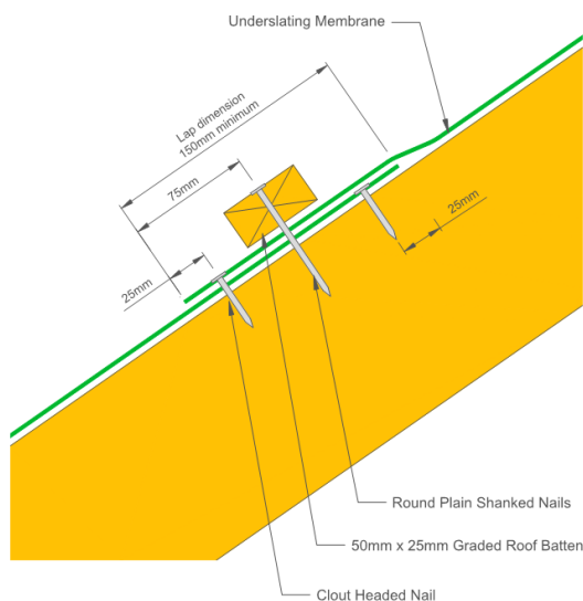
Figure 2: Creating the Overlap - Battened Overlap Detail
