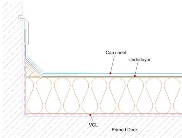
At all skirtings and upstands, the waterproofing should be at least 150mm above the level of the finished roof. Care must be undertaken not to bridge over any DPC or Cavity Tray positions.
