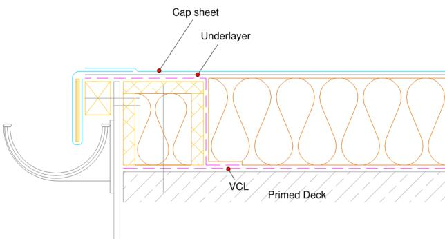
A welted drip edge should be formed wherever drainage to an external guttering is required. A plywood former should be introduced to form the drip. In warm roof build ups an insulated hard edge, 10mm thinner than the insulation thickness, should be incorporated.
