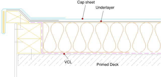
Check kerbs should be constructed to form a 50mm water check to prevent water from running over the edge incorporating a welted drip detail. In warm roof build ups a timber hard edge should be incorporated.
