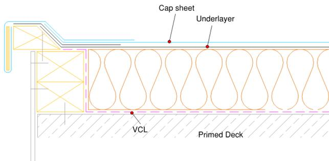
Check kerbs should be constructed to form a 50mm water check to prevent water from running over the edge incorporating a welled drip detail. In warm roof build ups a timber hard edge should be incorporated.
