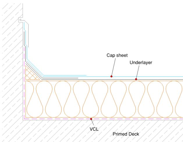
At all skirtings and upstands, the waterproofing should be at least 150mm above the level of the finished roof. Care must be undertaken not to bridge over any DPC or Cavity Tray positions.
