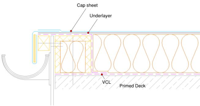
A welled drip edge should be formed wherever drainage to an external guttering is required. A plywood former should be introduced to form the drip. In warm roof build ups an insulated hard edge, 10mm thinner than the insulation thickness, should be incorporated.
