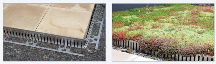
Where there is an exposed edge with no parapet, the perforated aluminium angle can be used to provide an edge to the green roof itself. It is recommended that the angle is mechanically fixed to the deck in some way. The pebbles are then installed the other side. This ensures free flow of drainage water.
