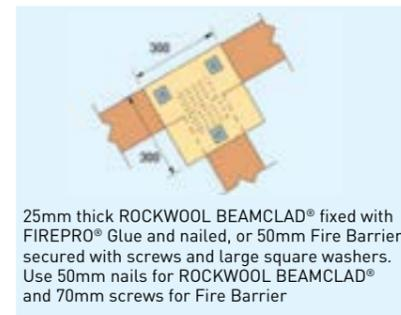
Figure 9 Nail plate protection
