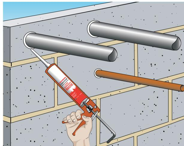
Figure 1 ROCKWOOL Acoustic Intumescent Sealant – Sealing around metal pipes
