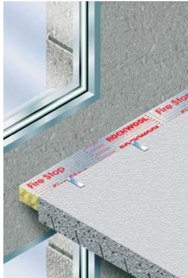
SP Firestop Slabs at floor / external wall junction
