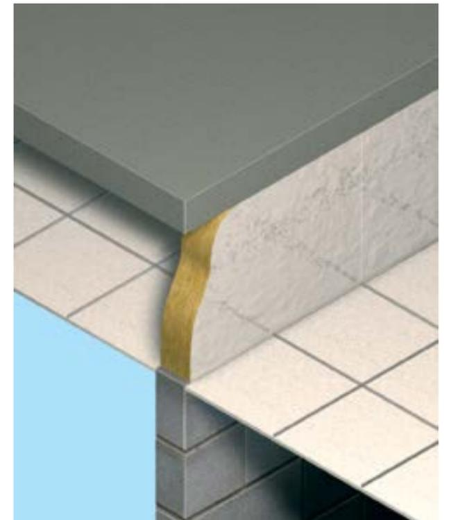
Figure 32 One hour Fire Barrier Slab – general view
