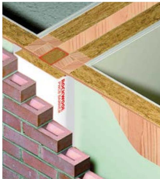
Figure 2 PWCB Cavity Barriers installed at separating wall position
