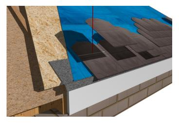
This image shows the build up of fascia, OSB sarking board, plastic eaves tray, the membrane should be taped to the eaves tray using a suitable weatherproof tape leaving at least 50% of the eaves tray exposed then the first two equal courses of slates which must overhang by 20mm.
