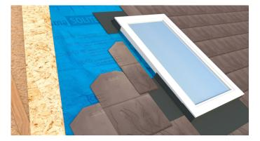
This image shows how **skylights** are flashed into the roof build up and slates just the same as you would with conventional slates. The skylight will have a flashing kit which is fitted in sequence with the slate rows.
