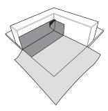
Apply the first flashing strip around the corner, forming an internal fold/ pleat.
