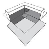
Apply the second flashing strip up to the corner.
