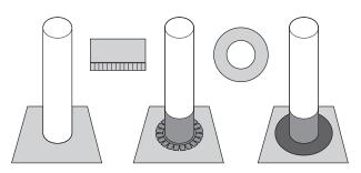
Cut the flashing strip into a series of 'tongues' (approx. 30 mm wide). Take the strip around the pipe and press the tongues down onto the roof surface.
