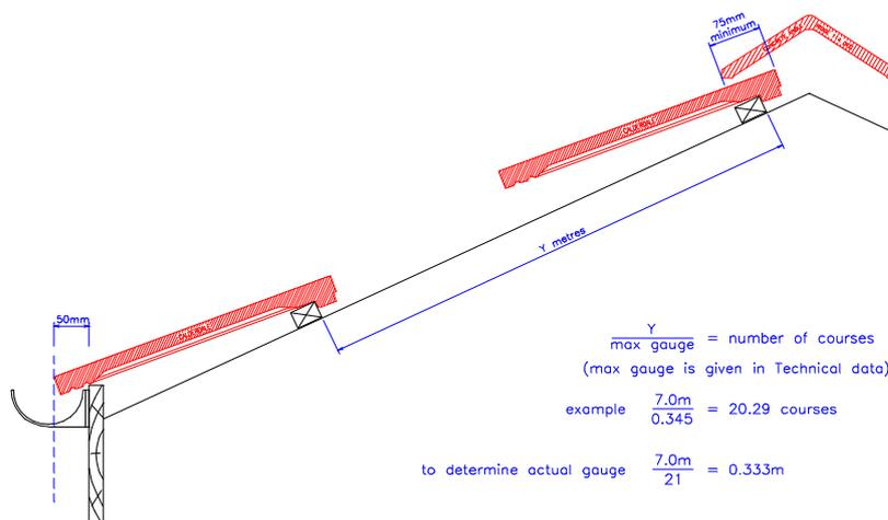
In our example this works out at 20½ courses, therefore 21 courses will be required. The distance as measured between the first and last batten is then divided by 21 to determine the actual, setting out gauge.
