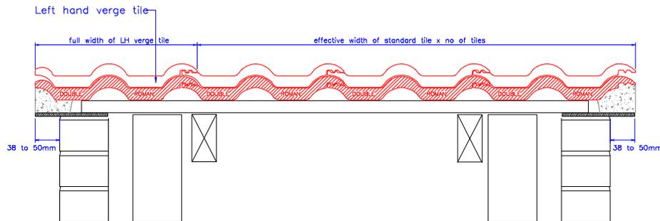
Most roofing tiles have some adjustment in their linear coverage, often around 3 to 6mm. So some flexibility in setting out is possible to avoid having to cut tiles at one or both verges. When using traditional bedded verges the overhang can also be adjusted between 38 and 50mm to suit the tiles.
