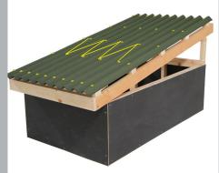
Nail every corrugation along of the eaves, either side of the vertical laps and every other corrugation on the intermediate purlins in a offset pattern.
