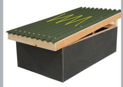
Nail every corrugation along of the eaves, either side of the vertical laps and every other corrugation on the intermediate purlins in a offset pattern.
