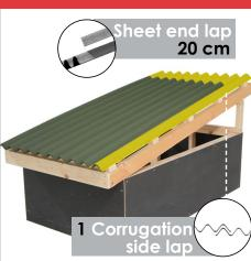
Lay the sheets with: 20cm sheet end lap Single corrugation side lap
