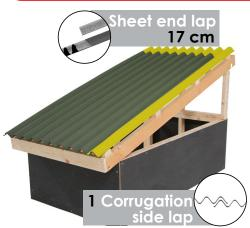
Lay the sheets with: 17cm sheet end lap Single corrugation side lap
