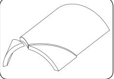
**2.** Drill one Ø 5mm hole (A) 80mm from the point of the cut edge. Drill a second hole (B) 180mm from the uncut edge of the tile.
