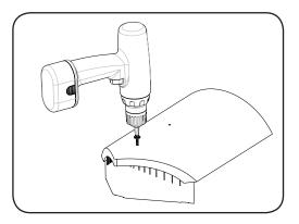
7. Fix the tile to the roof through hole (B), using the screw found in the Manthorpe GDRH roll-out hip kit or a suitable fixing.
