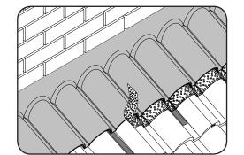
**7.** Using a sharp knife, cut away any excess flash vent which is protruding from the front edge of the lead.
