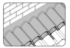
**6.** Dress the lead over the flash vent and tiles using standard lead working practices as recommended by the L.S.A. Ensure that the lead is dressed down beyond the upper indicator line of "trim to suit lead" moulded on the vent.
