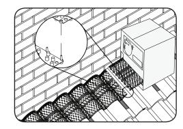
**5.** At the end of the abutment cut off any excess roll with a sharp knife. If one roll is not sufficient to complete the run of the abutment then additional rolls can be joined together by clipping the end of one roll to the start of the next as shown in the image above.
