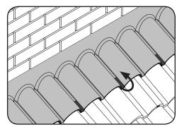
**8.** Finally, bend the clips over the clips over the lead ensuring that they are firmly pressed into position (any excess clip may be trimmed to length).
