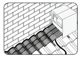
**4.** Moving across the roof from left to right, roll the flash vent out onto the tiles removing the backing tape from the mastic strip and firmly pressing it down onto the tile profile as you go.
