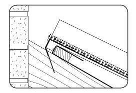
**3.** Tear open the perforation at the base of the box and pull out the start of the roll. Position the long pins against the back face of the top row of tiles as shown in the image above.
