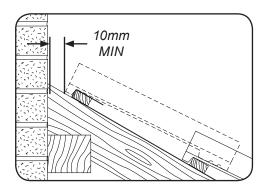
**1.** To achieve the required 5mm<sup>2</sup> air flow, fit the top roof batten to provide a 10mm gap between the back of the top row of tiles and the wall. The felt must then be returned around the top batten.
