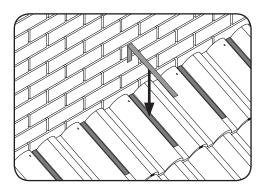
**2.** Remove the backing tape from the clips provided and hook the over the top row of tiles at 300mm centres (ensuring that the tiles are clean and dry). Bend the short leg of the clip round under the batten. Additional clipping may be required depending on the level of exposure as per Lead Sheet Association (L.S.A.) recommendations.
