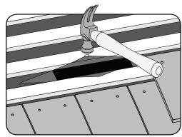
**4.** Fold the top tab tight up against the batten above it and secure it in position with a staple or tack.
