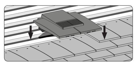
5. Slot the vent into the position. Make sure the spigot passes fully through the felt so it is accessible from the loft space. On roofs with smaller batten gauges it may be necessary to flex in the spigot clip to allow it to pass through the opening. Slide the vent left or right to align it with the adjacent tiles.
