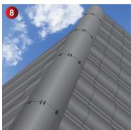
Continue this process along the ridge to the end. Secure the ridge end tile through the pre-drilled holes provided or drill a hole through when using reclaimed tile.
