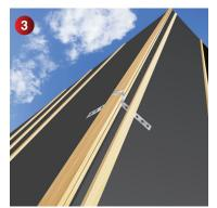
Install the top tiling batten as normal, leaving a 10mm air gap.
