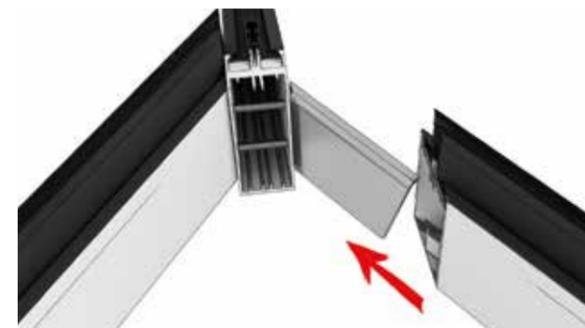
**7** Slide the hip rafters over the pre-fitted hip brackets as shown. If a central bell rafter is specified, hip brackets will not be installed and instead the ridge will be slotted. See 'Bell rafter installation' prior to continuing.
