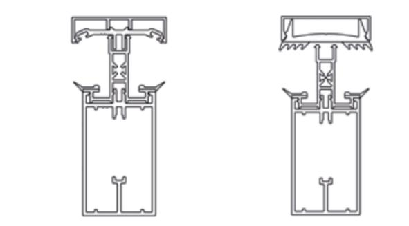
**22** Fit hip and transom pressure plates **centrally on the rafter** (hips will locate into the central channel on the rafter). Ensure that pressure plates are pushed up against the side of the ridge topcap.
