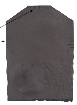
**Nails:** Eco Slates must be secured using the relevant size, copper, stainless steel or hot-dipped galvanised nails with a minimum head diameter of 5mm.
