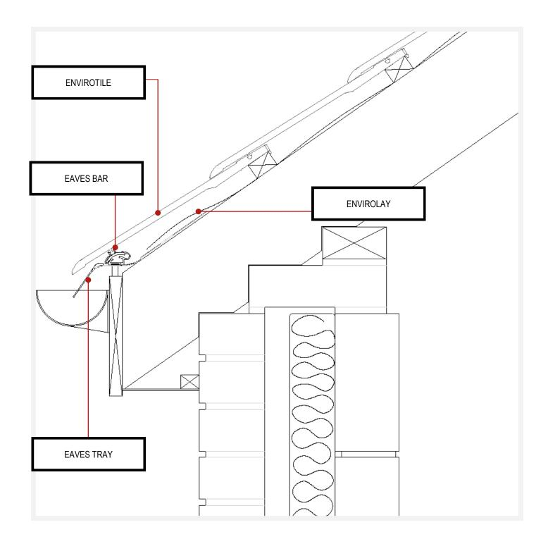
Approved Document F2 (1995) Building Regulations and BS5250:2002 'Control of Practice for Condensation in Buildings' detail the requirements and practicalities of minimising condensation. Condensation must be managed in order to prevent damage to the thermal and structural properties of the materials used in the roof eaves prevent rain from damaging the building walls and ensures effective collection and release of run-off.
